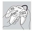
By holding the controller like this, you can operate the Control Stick freely with your left thumb. Using your right thumb, you can easily access the A-, Bor C-Buttons.
